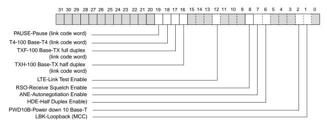
\*The software reset bit (bit0 of CSR0) has no effect to this register.
